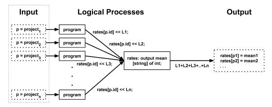
Fig. 3. Overview of the semantic model provided by *Boa* for the query in Figure 2. Each project is a single input and fed to a single process. Each process sends messages to the output process. The output process produces the final result. Each solid box represents a logical process.
