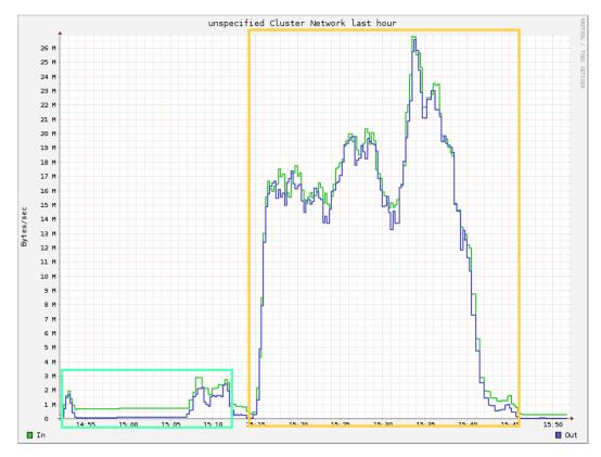
Fig. 26. Network utilization. Note the minimal use by the MapFile store (left) compared to the HBase store (right).
