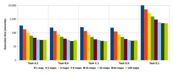
Fig. 22. Scalability of sample programs. Y-axis is total time taken. X-axis is the number of available map slots in the cluster. NOTE: y-axis is in logarithmic scale.
